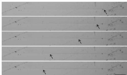
(a) The first one is photograph before the loading event-1, and the following four photographs are the one after the loading event-1, 2, 3 and 4 in table 3
