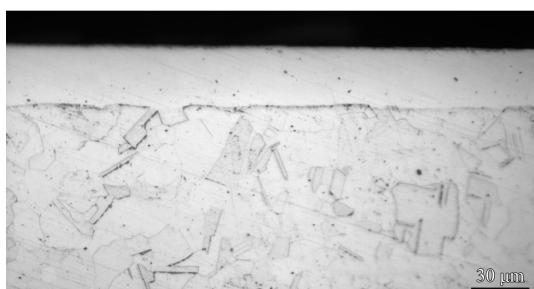
(b) Electro-etched by saturated oxalic acid solution
