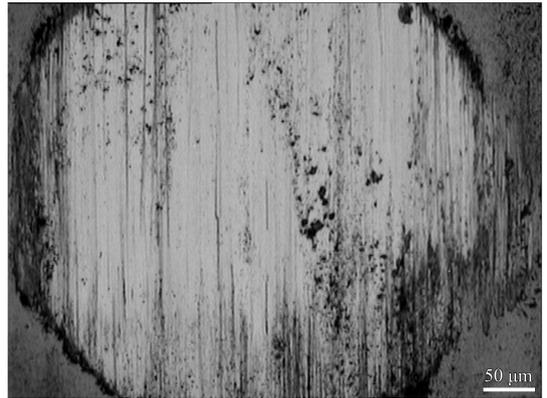
(b) 5 N,  $\text{Al}_2\text{O}_3/\text{MoS}_2$  composite coating
