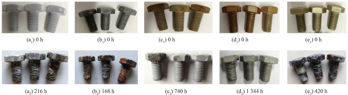
(a) Al films (b) Cyanide zinc plating films (c) Al films treated by chemical conversion (d) Al films treated by blasting and chemical conversion (e) Cyanide zinc plating films treated by passivation
