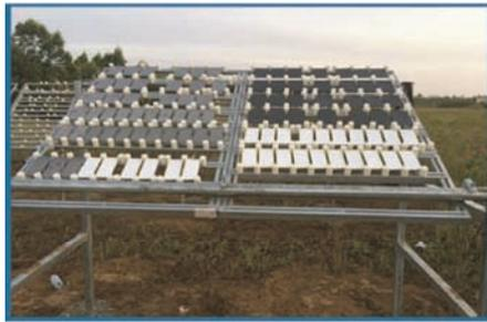
(a) Corrosion experiment station at Wenchang Base
